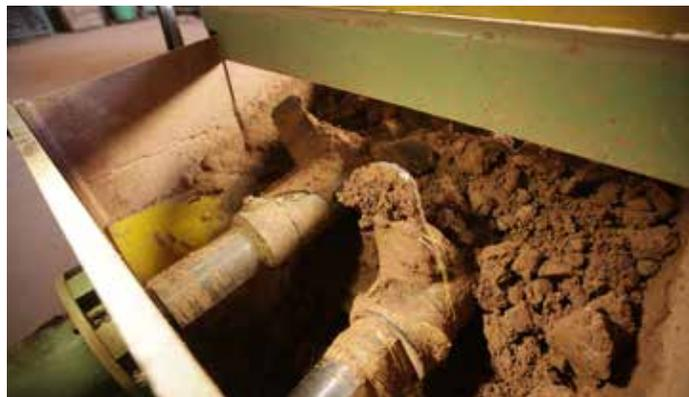
**FIGURA 3:** PROCESSO DE MISTURA DA MASSA CERÂMICA.
